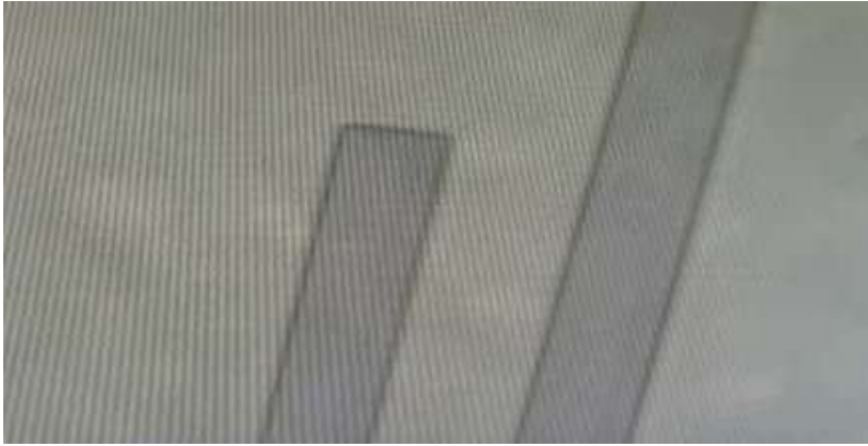
Figure 5: In this microscope image of the developed photoresist pattern, the features turned out well.
