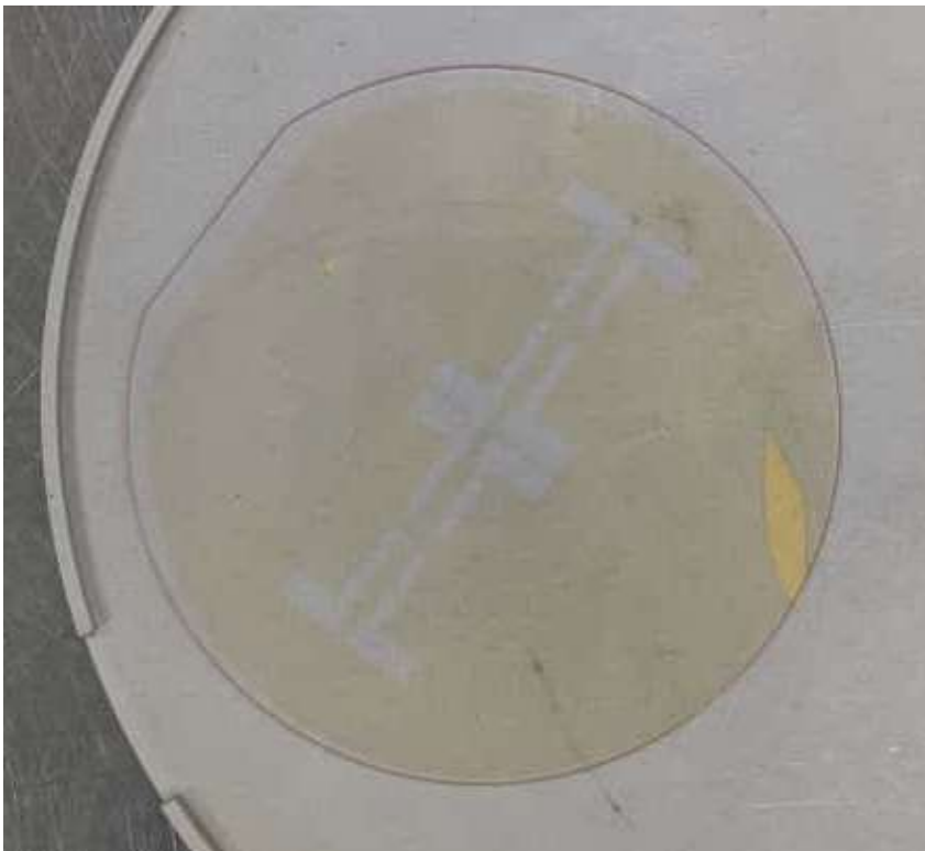
Figure 4: The features are clearly visible in this photograph of the photoresist pattern following development.
