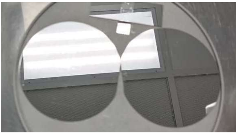
Figure 6: sputtering deposition leaves a thin and smooth layer of Pt coating the surface.
